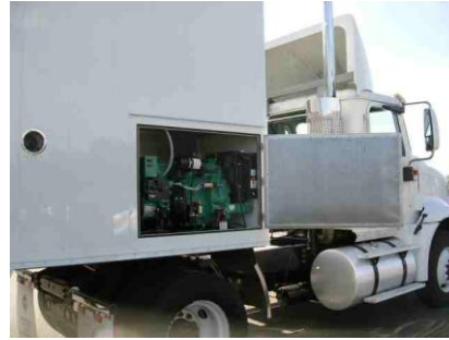
Figure 44—MSU Power Supply (Diesel Generator)
